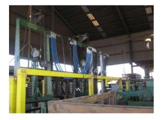
Note: Drape Hose conversions are designed for Loader/Unloader towers with mechanical #: 307.210. & .218. series, (UL20, UL26 & UL37).
